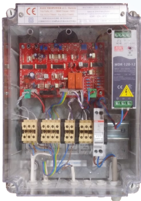
Batteries monitor BM1
